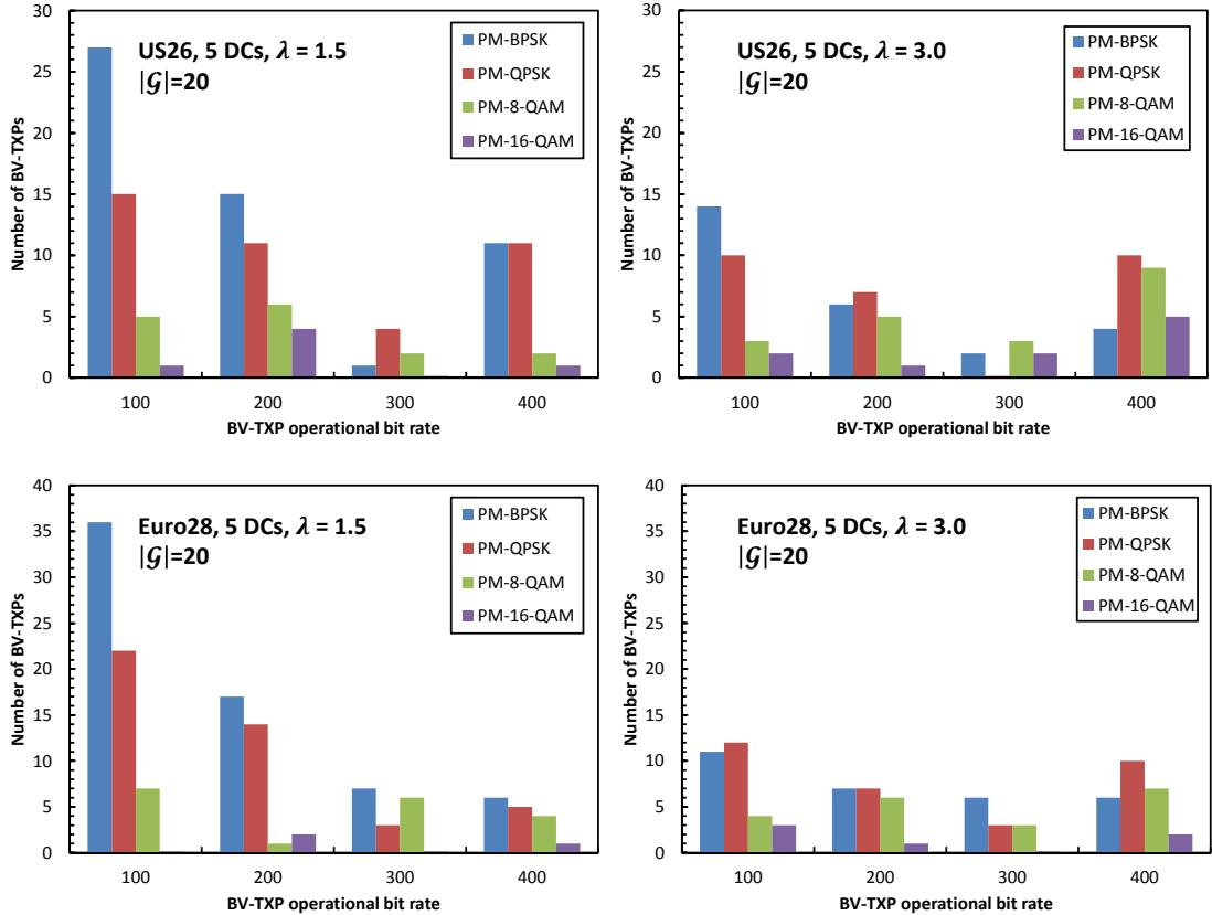
Figure 8. Operational bit rate and modulation format employed by the BV-TXP equipped in US26 (top row) and Euro28 (bottom row) networks with 5 DCs. Scenarios with  $\lambda=1.5$  and 3.0 are considered.
