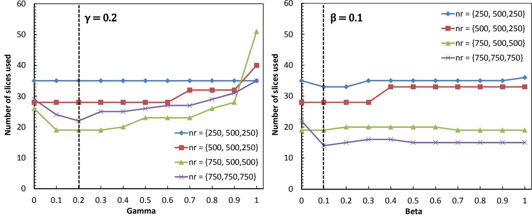
Figure 7. Number of slices used in the INT9 with 3 DCs using CPRMSA-PD: with parameter  $\beta=0.0$  and different values of parameter  $\gamma$  (left); with  $\gamma = 0.2$  and different values of parameter  $\beta$  (right)
