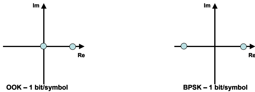
Figure 6-3: Constellations that use only the real part of the field and carry 1 bit per symbol.
